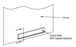
labor costs. The best way to figure out how many segments you need is during the testing phase of the design. Place a few 1" pieces of gasket around the perimeter of your box. Run a baseline test and then add and subtract gasket pieces until you find the optimal number. This also allows you to upgrade by adding a few more pieces if you later need to meet more stringent requirements or the frequency of your internal electronics goes up in subsequent product modifications.
